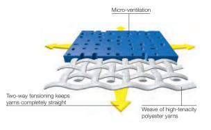
Made using the exclusive patented Précontraint® Ferrari® technology, Soltis® textiles are maintained under tension throughout the whole manufacturing cycle.
